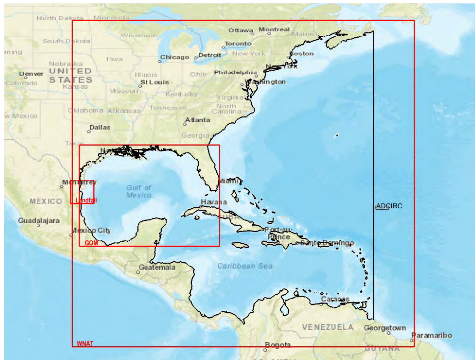
Figure 21. Map showing the three grid boundary extents for the regional wind and pressure fields in (red) and the ADCIRC model domain shown in black. Note, the Landfall domain is track dependent and not fixed in one location.
