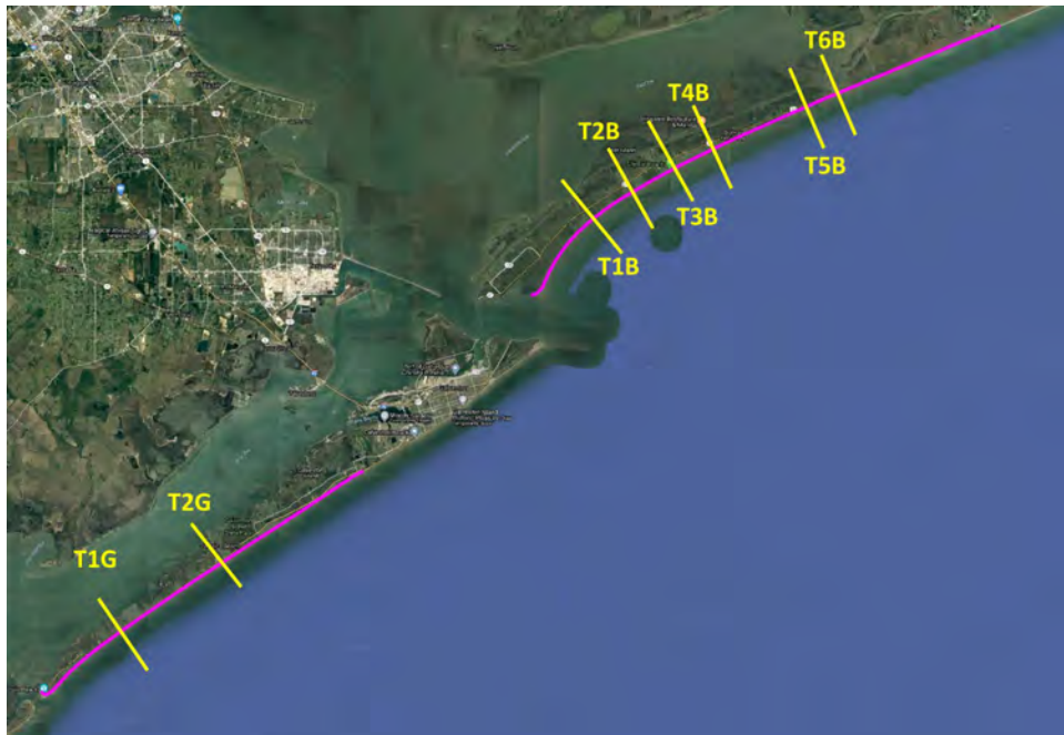
Figure 40. Hazard transects T1G and T2G with 1% AEP SWL in ft, NAVD
